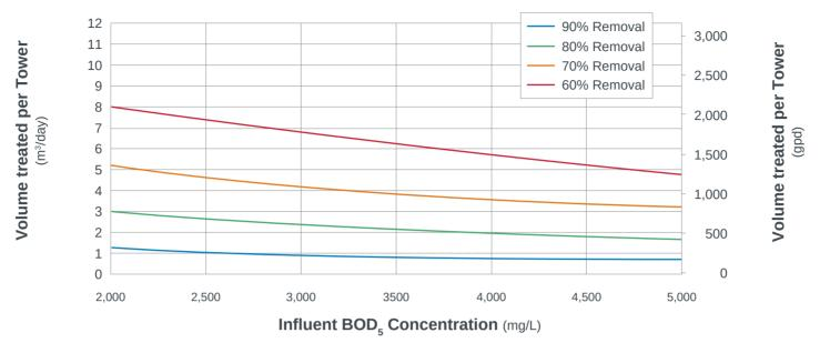
This performance graph is to be used as a sizing guide only. Actual performance is determined by site specific factors and may vary. The above information is based on the following; a continuous flow system; brewery wastewater and water temperature at 86°F | 30°C. Removal rates and reductions are based on soluble BOD only. BioGill and its authorized representatives do not guarantee performance unless stated otherwise.
